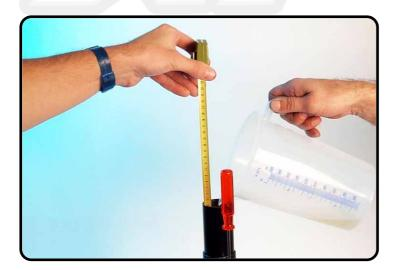
Adjust oil level about 45mm under the edge of the tube and set compression adjusting knob on position 1.
