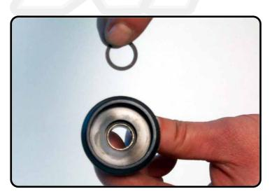
Assemble the back-up ring.
