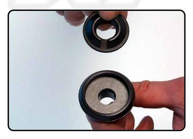
After assembly the rebound rubber, check if the rubber can be rotate in the holder.
