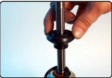
Should it be the case to assemble spacers, then place them with the flat side direction rebound rubber.
