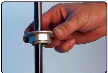
Remove the steel washer and springring.
