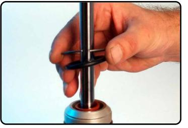
Remove the circlip and O-ring.
