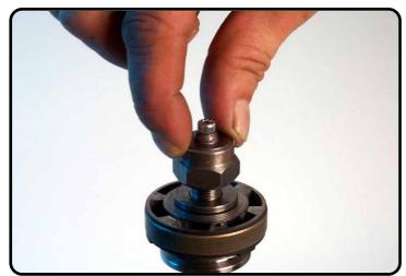
Screw the piston-rod nut on piston-rod....
