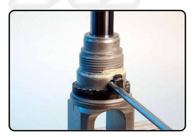
Place T107S through mounting fork / eye under the needle and adjust position ring in the highest position.
