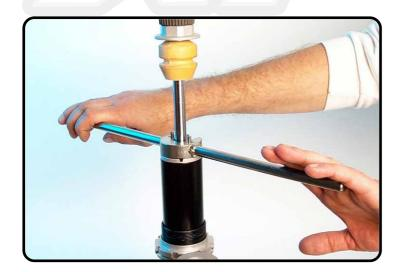
Tighten the screw-cap with T125S.
