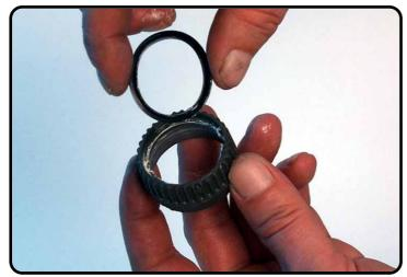
Assemble the adjusting knob and turn the knob to position 1.
