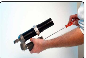
Push the separation piston downwards, and hold the tube side in a angle. (about 45 degrees) Repeat those procedures several times.
