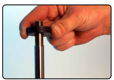
Remove (should this be the case) the spacers. Pay attention to the assembling direction!!!
