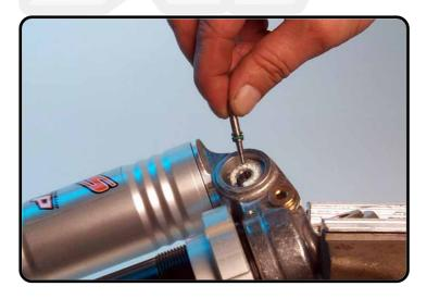
Screw the adjusting needle hand tight into mechanism.
