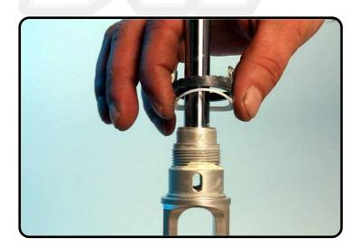
Replace the seal and the position ring.
