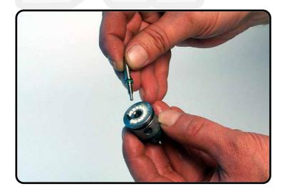
Assemble mechanism without adjusting needle. (left handed thread)
