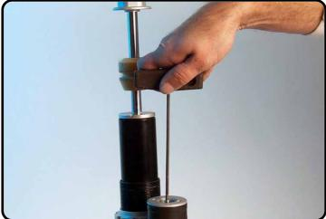
Unscrew the screw-cap with T125S.
