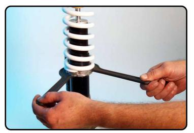
Tighten the spring retainers with T106.
