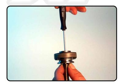
Place a screwdriver on top of the pistonrod and remove the entire assembly.
