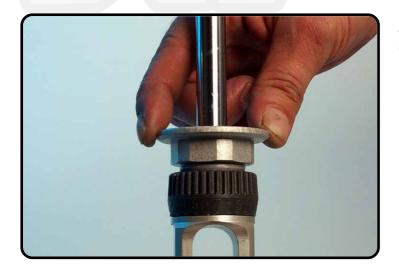
Assemble the steel washer and springring.
