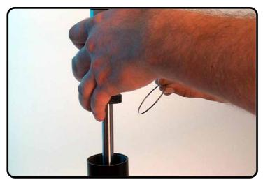
Slide piston-rod "complete" into the tube and assemble the springring above the piston in the groove with support of...
