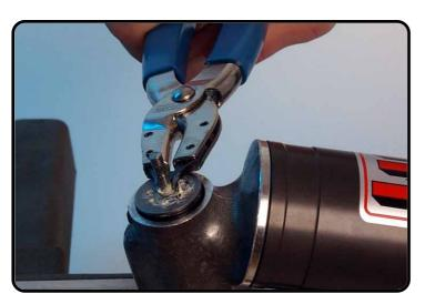
Lift out the compression control mechanism.
