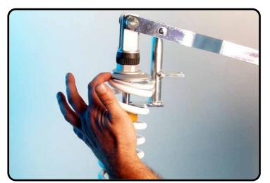
Assemble the open spring retainer with T101S. Closed side of the retainer on the end of the coil.
