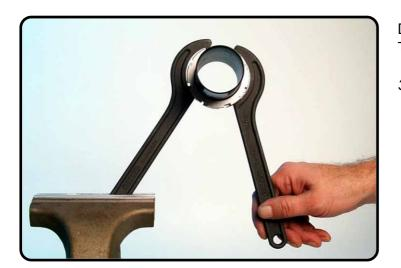
Disassemble the spring retainers with T106.
