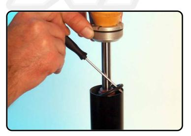
Lift the O-ring out of the tube.
