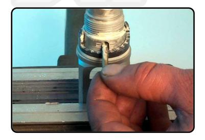
Grease the ring and pin with T159 and assemble the pin.
