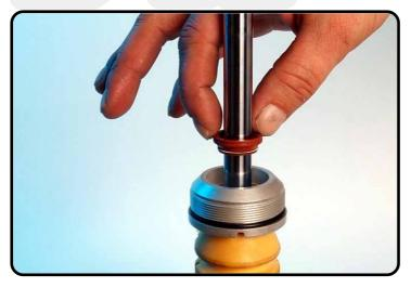
Grease the innerside dirt scraper with T625 and assemble.
