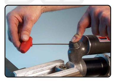
Push adjusting knob with the spring directly on the steel ball and tighten Allen screw.
