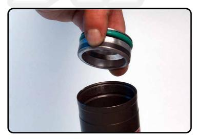
Assemble separation piston (with piston-ring) always into direction of the screw-cap.
