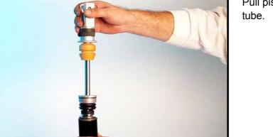
Pull piston-rod "complete" out of the tube.
