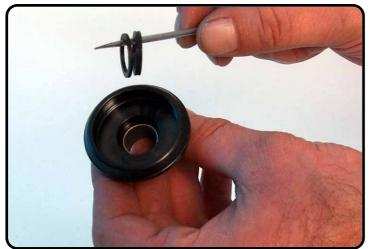
Remove the quad ring and back-up ring.
