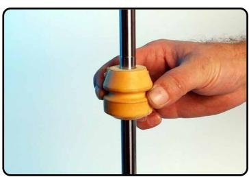
Assemble the screw-cap.
