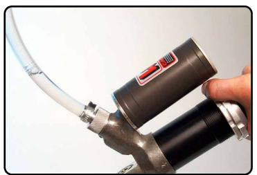
Cant to a view times the shock absorber and repeat the procedures several times until all air is bled out.
