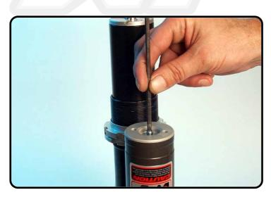
Place the shock absorber (reservoir) in T170S and fill it with nitrogen ( $\pm$ 20 sec.) and tighten the plug under pressure.
