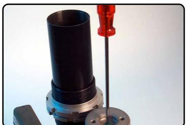
Push the separation piston with T107S to the bottom and slide O-ring as far as the screw-cap.
