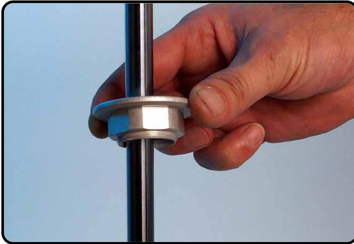
Remove the circlip and ring. (On picture with nut)
