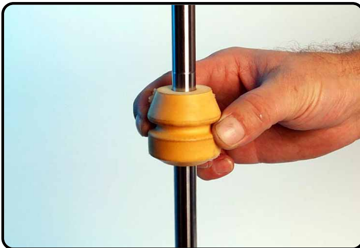
Assemble the bump rubber.
