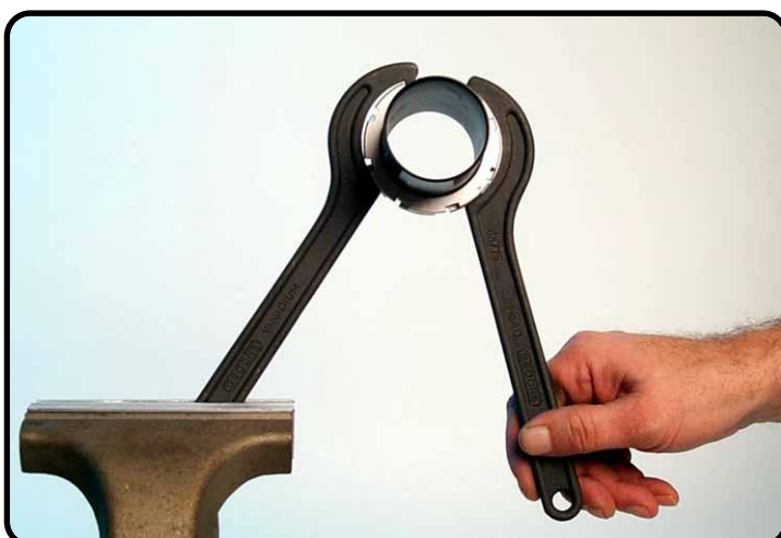
Disassemble the spring retainers with T304.
