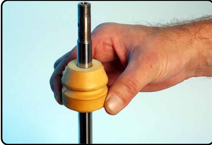
Remove the bump rubber.
