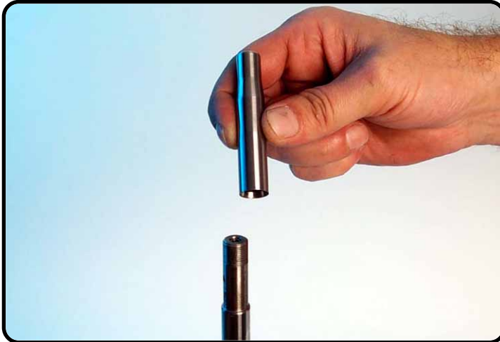
Place T313 on top of the piston-rod.
