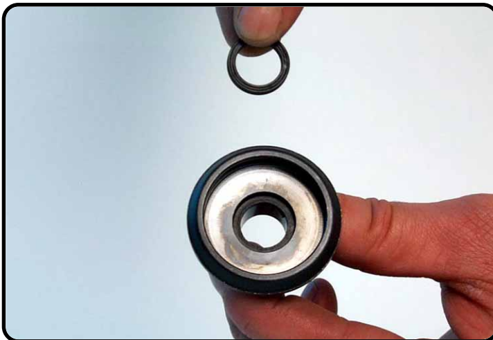
Assemble the quad ring.
