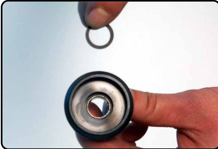
Assemble the back-up ring.
