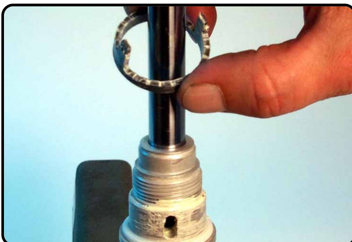
Remove the position ring.
