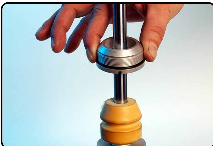
Assemble the screw-cap.
