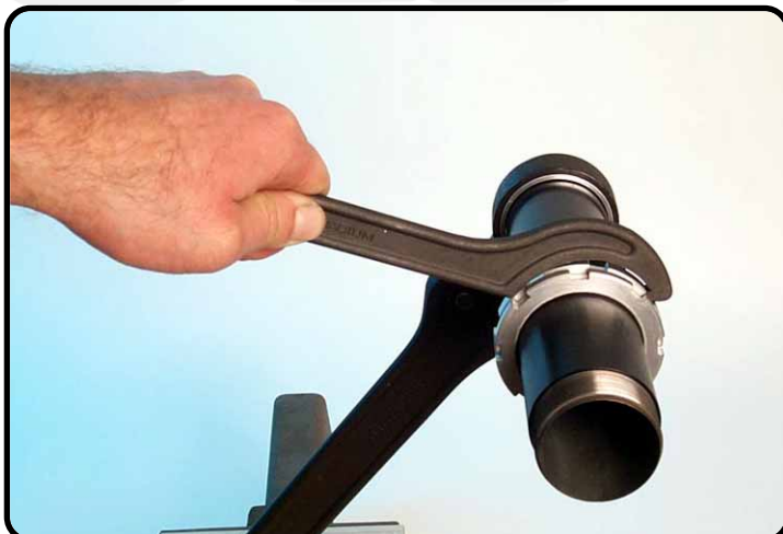
Unscrew threaded bush with T304.
