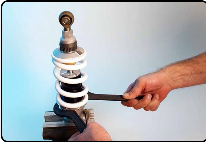
Tighten the spring retainers with T304.
