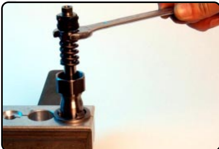
Unscrew the rod tap. (size 17)
