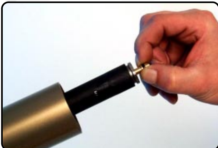
Pull the cartridge out of the forkleg.
