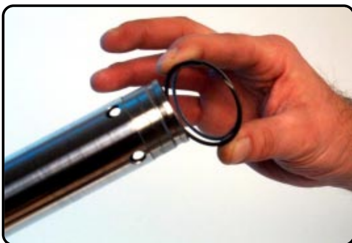
Remove the spacer ring and circlip.
