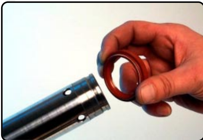
Remove the oilseal.
