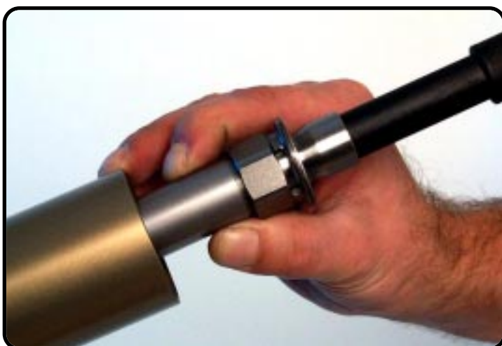
Remove the cartridge.
