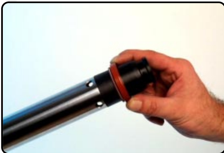
Slide the oilseal over the inner-tube.
