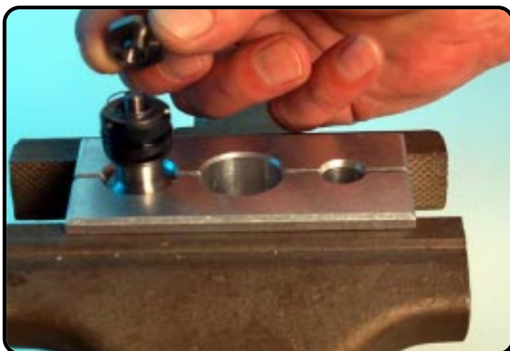
Remove the check-valve nut.
