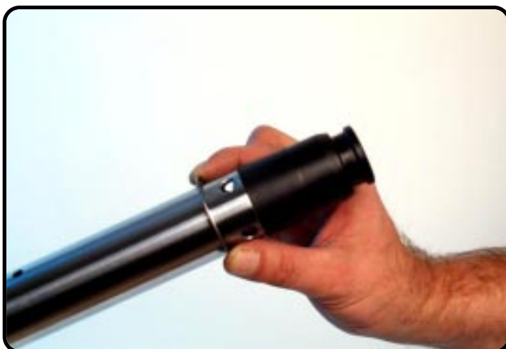
Replace the support ring.
