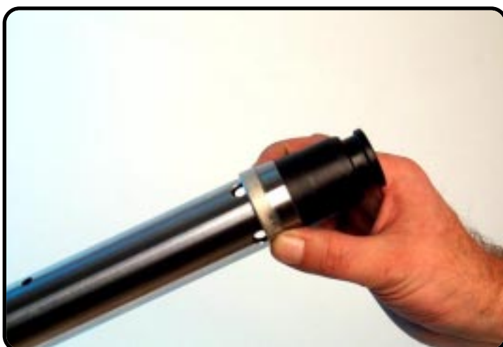
Assemble the DU-bush outer-tube.
