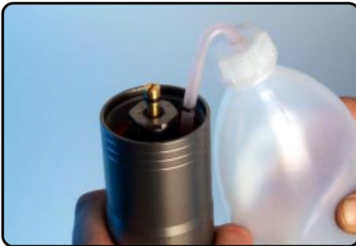
Hold the upper side of the piston rod exactly level with the (fully compressed) outer-tube. Remove the oil till the correct level.
