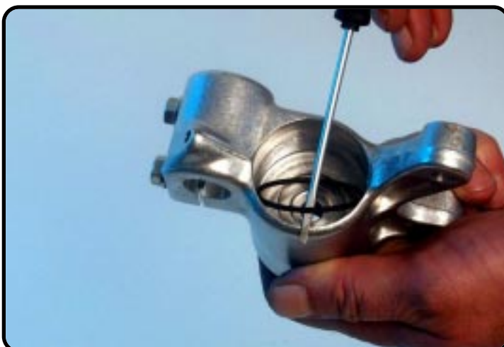
Lift the O-ring out the groove of the axle-clamp.
