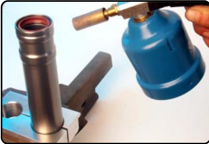
Heat the outer-tube near the oilseal.
