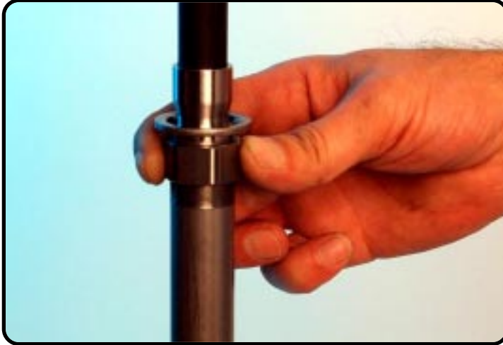
Assemble the screw sleeve on the tube.
