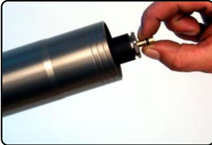
Pull the cartridge out the forkleg.
