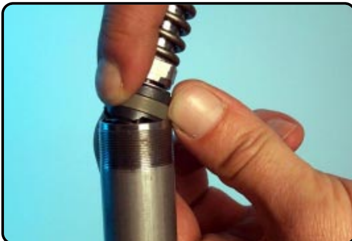
Assemble the piston-rod "complete" with piston ring into the tube.
