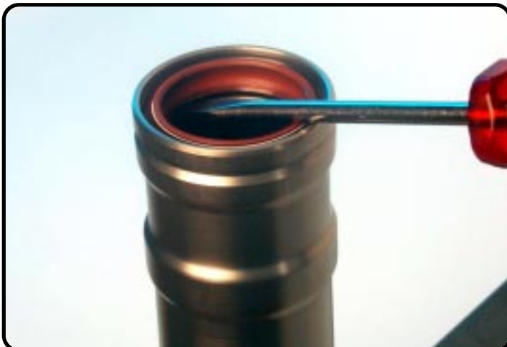
Pitch a screwdriver just below the oilseal...
