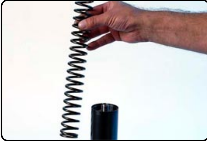
The spring out of the forkleg.
