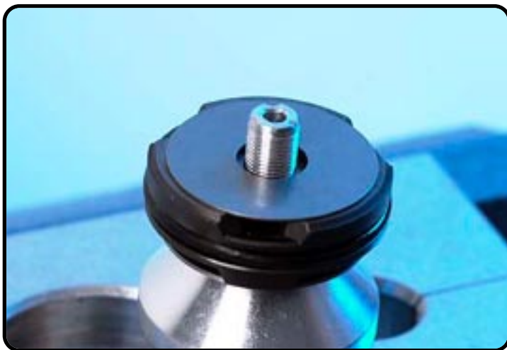
Assemble the shim(s).
