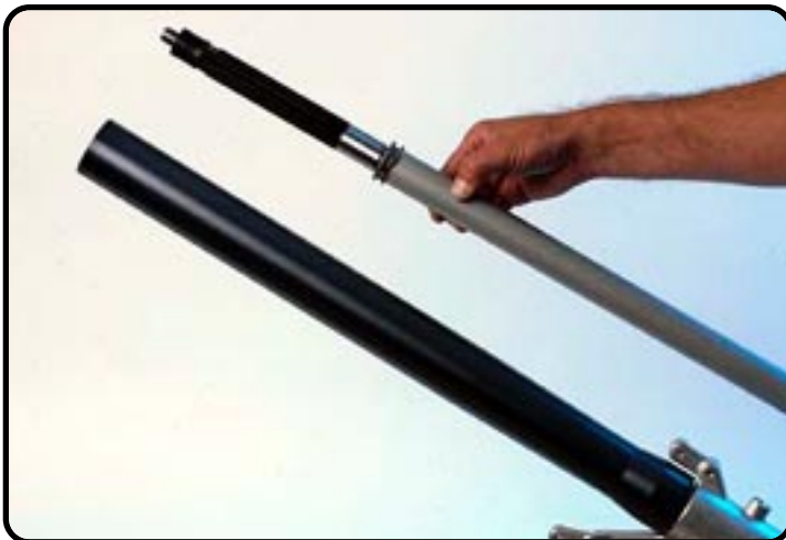
Cartridge out of the forkleg.
