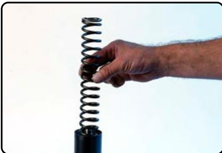
Remove slowly the spring out of the forkleg.
