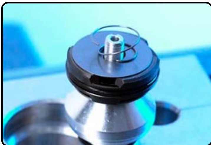
Assemble the spring. Pay attention to the assembling direction!!!
