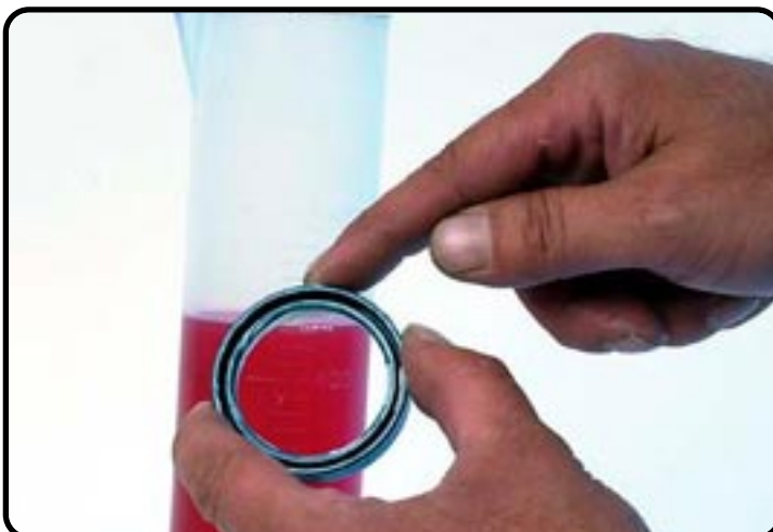
Grease the outside of the oilseal with frontfork oil.
