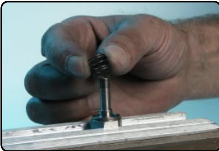
Temove the check-valve spring.
