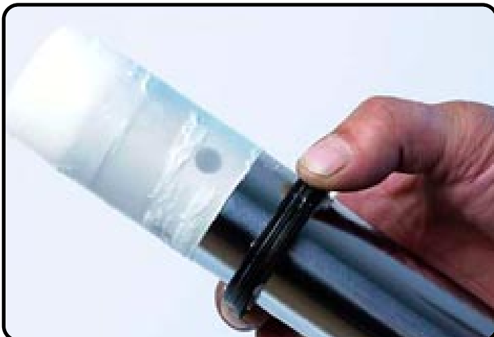
Slide the dirt scraper over the inner-tube.
