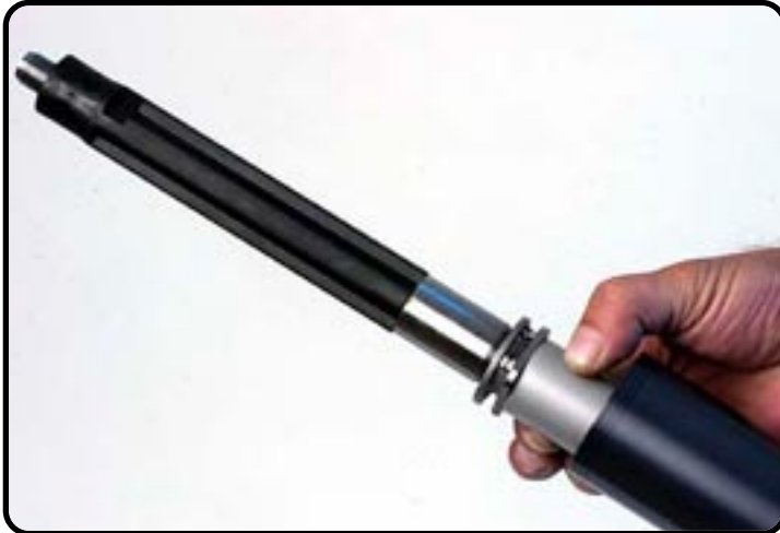
Remove the cartridge out of the forkleg.
