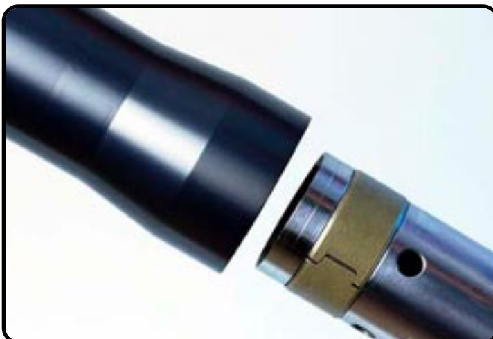
Slide the outer-tube over the inner-tube.
