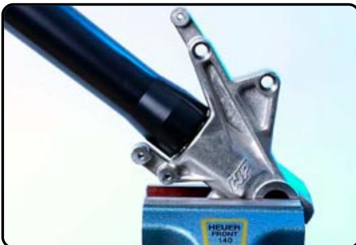
Clamp the axle-clamp like picture in the vice.
