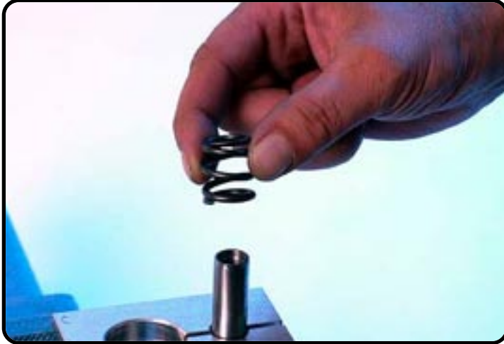
Remove the rebound spring.
