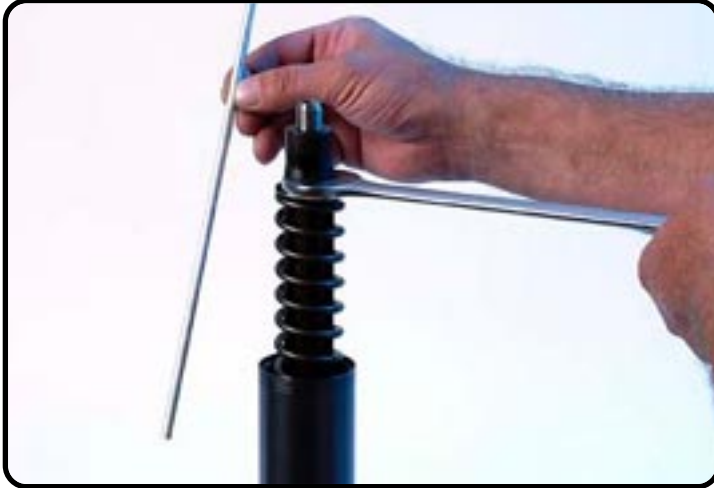
Adjustment tube out of the piston-rod.
