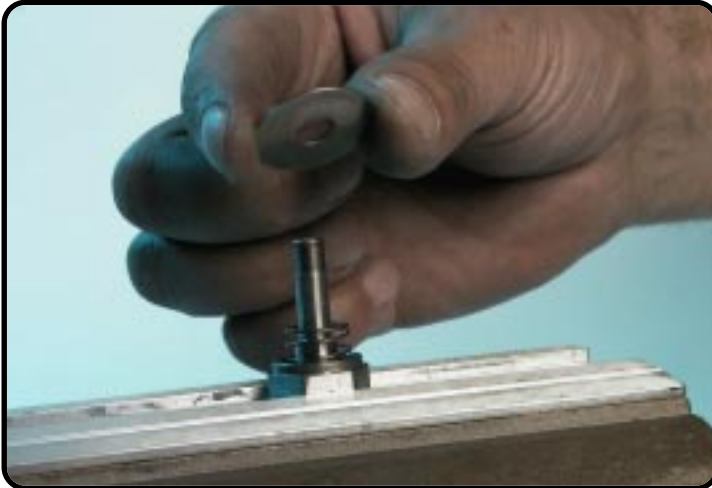
Remove the chek-valve shim(s).
