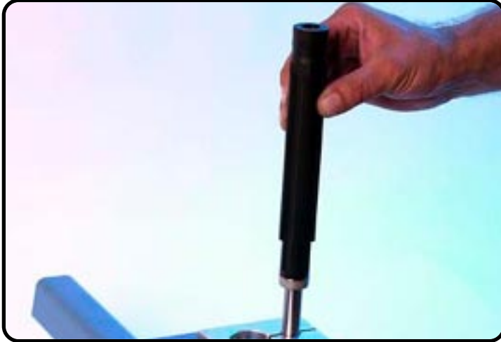
Turn the hydraulic stop of the piston-rod.
