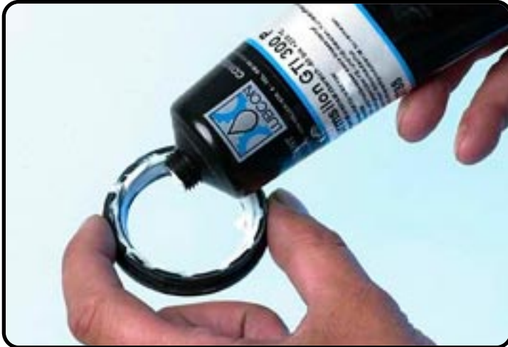
Grease the innerside of the dirt scraper with T511.
