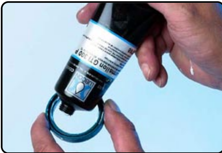
Grease the innerside of the oilseal with T511.
