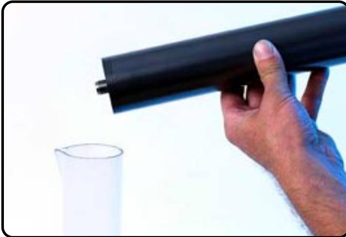
Drain the oil out of the forkleg.
