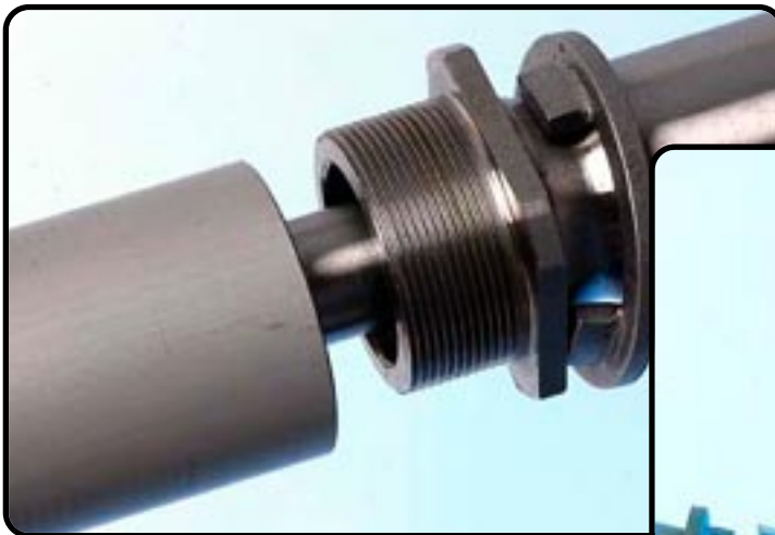
Wet the thread of the screw sleeve with T131.
