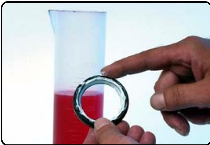
Grease the outside of the dirt scraper with frontfork oil.
