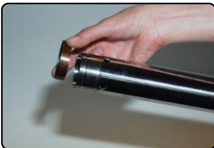
Remove DU-bush outer-tube.
