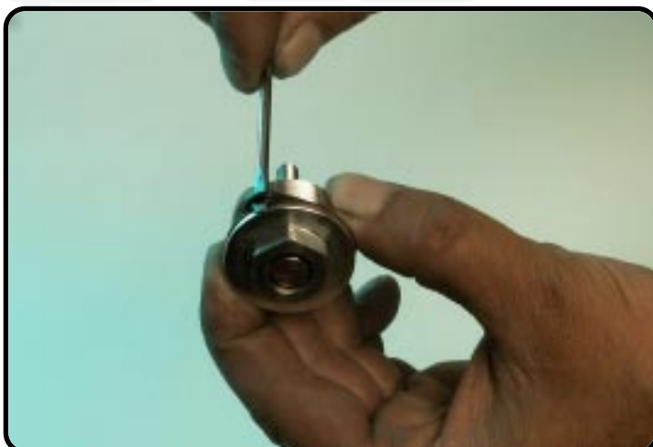
Disassemble the O-ring.
