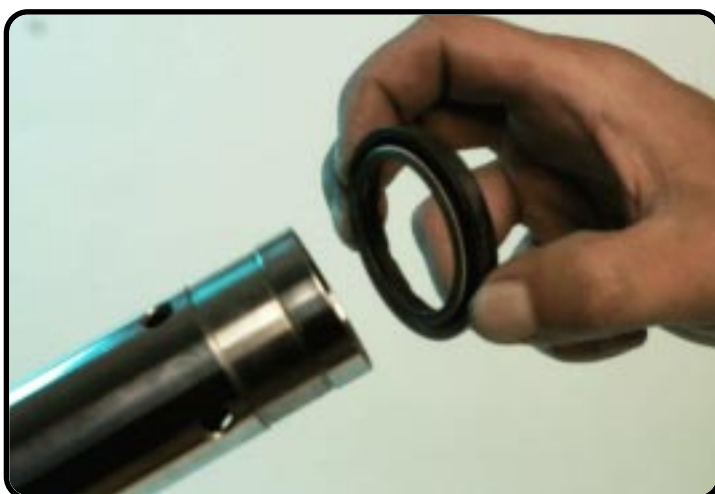
Remove the dust wiper.
