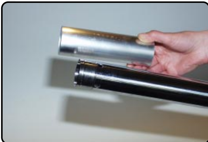
Remove DU-bush inner-tube.
