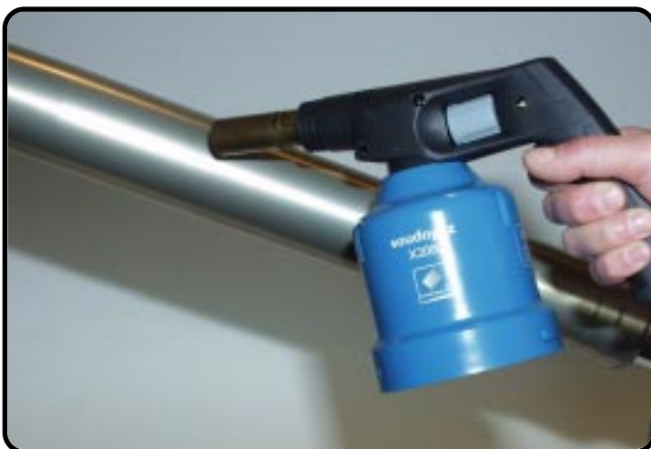
Heat the outer-tube at this level..
