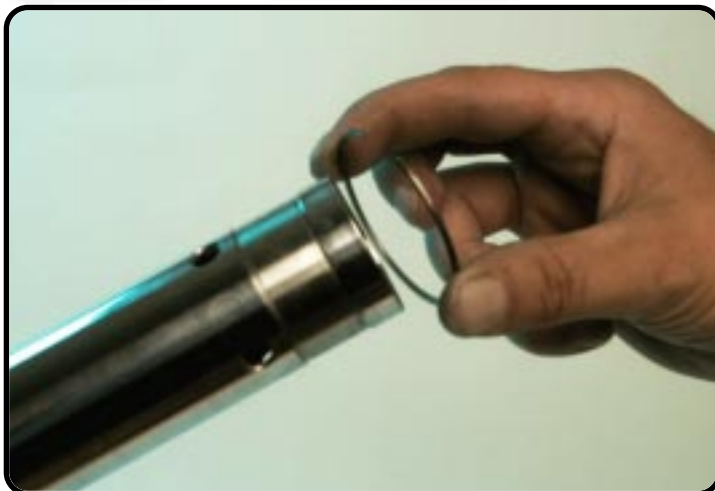
Remove the circlip.
