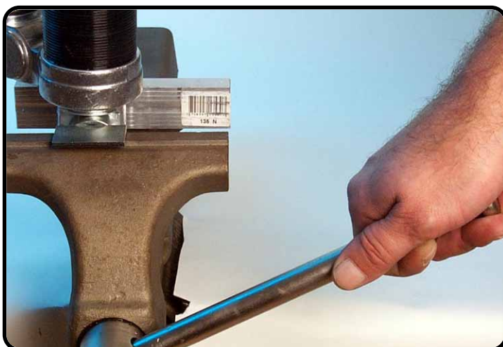
Press the heim-joint KGW out of the bottom with the vice.
