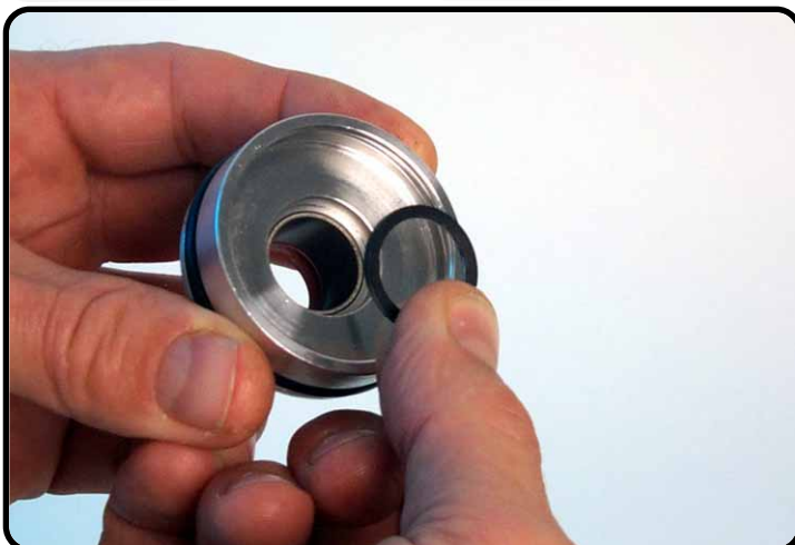
Assemble the back-up ring.
