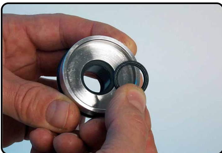
Assemble the quad ring.
