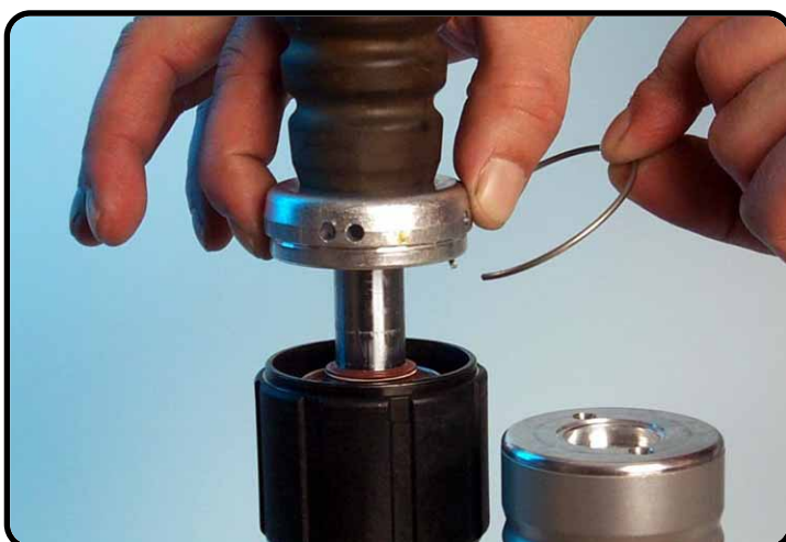
Assemble the springring also past the groove.
