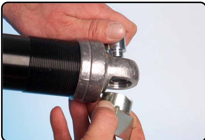
Disassemble heim-joint KGW with T1207S.
