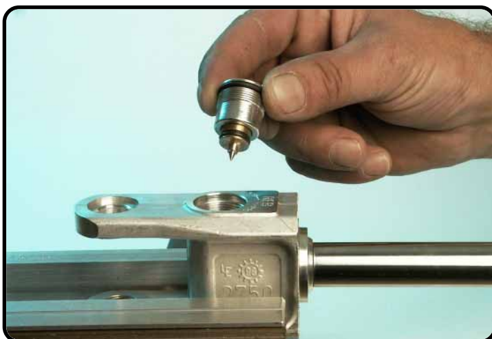
Disassemble the adaptor out of the mounting fork with a screwdriver.
