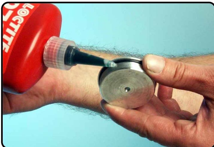
Drip T132 on thread screw-cap.
