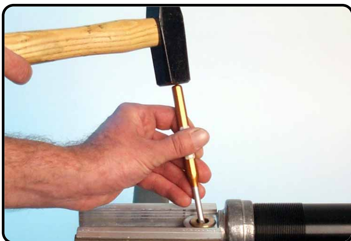
Tap adaptor bushes out of the heim-joint and remove the seals.
