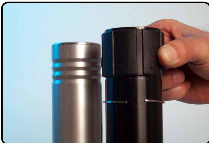
Slide guide over the springring.
