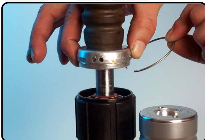
Assemble the springing.
