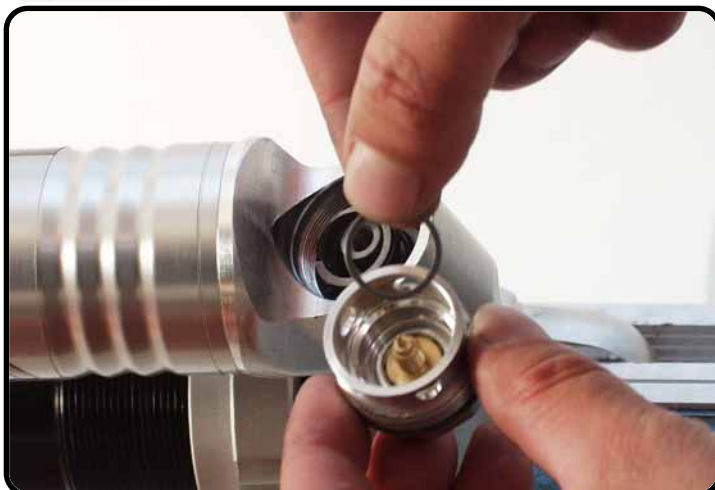
Place the ring into the screw-cap.
