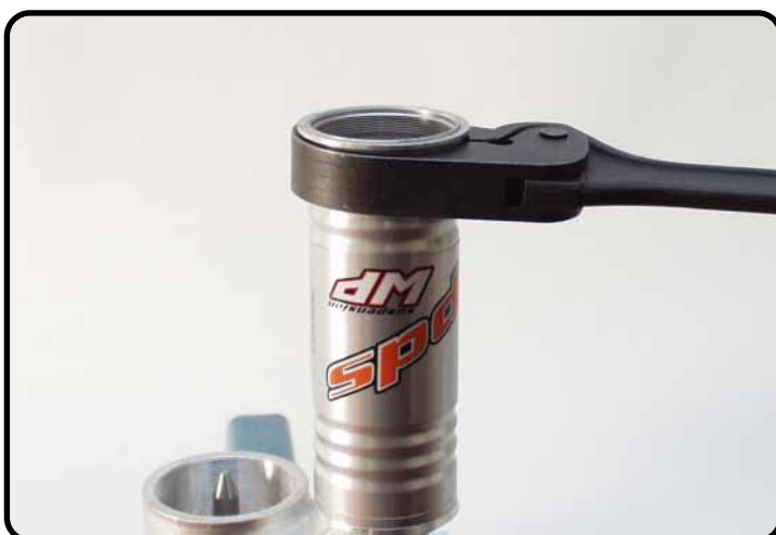
Unscrew the reservoir from the bottom with T146 and bush T147.
