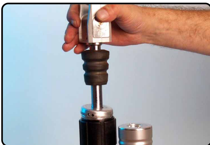
Pull the piston-rod fully out.
