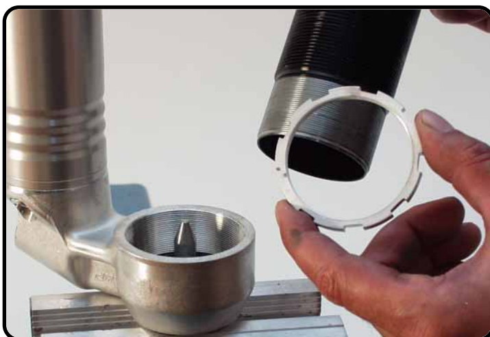
Screw the lock retainer of the tube.
