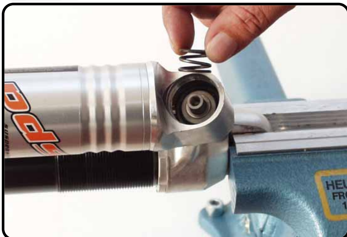
Remove the spring.
