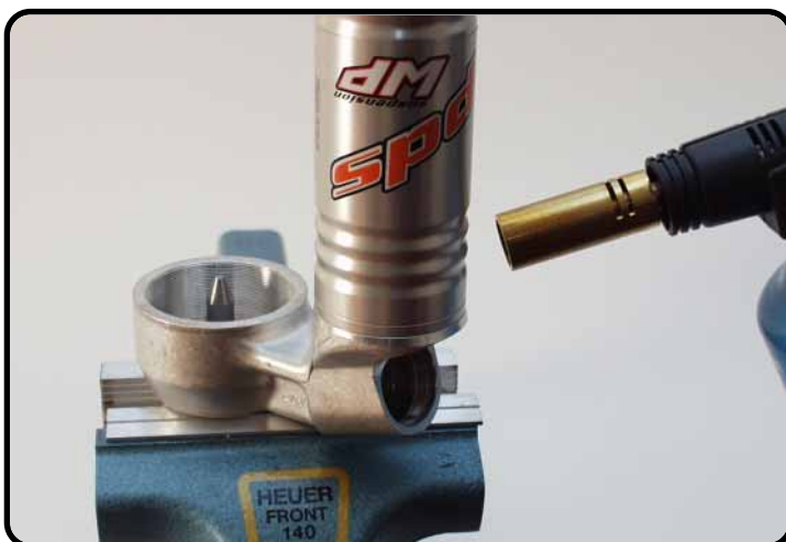
Heat the reservoir near the bottom.
