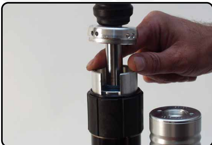
Push the adaptor DU-bush downwards.
