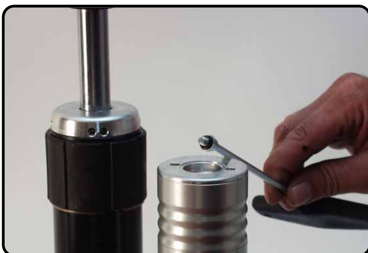
Nitrogen plug with O-ring.
