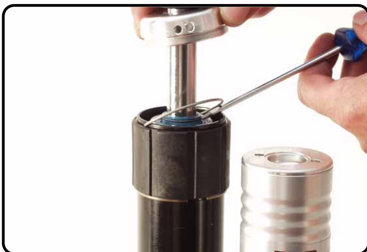
Disassemble the springing out of the tube.
