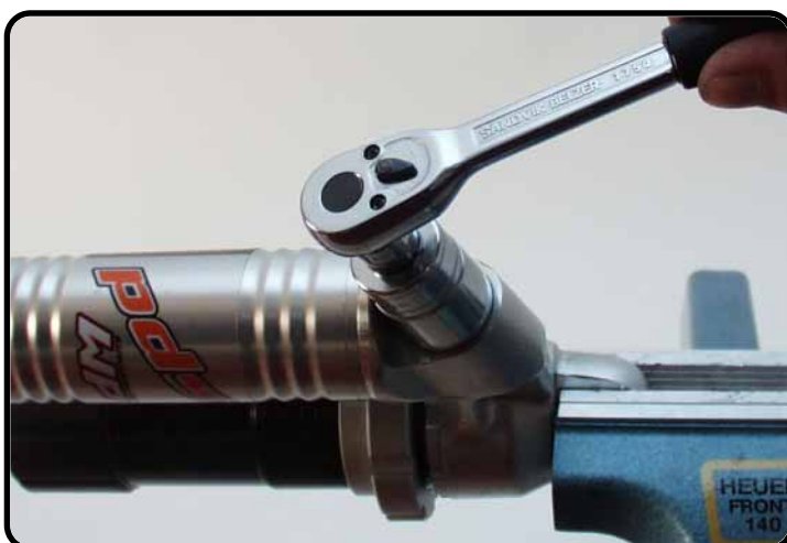
Tighten the screw-cap.
