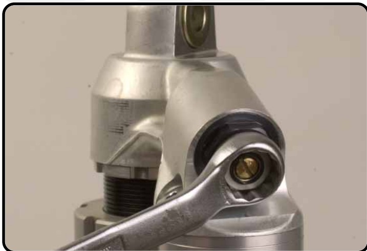
Compression High-Speed position (DCC)!
