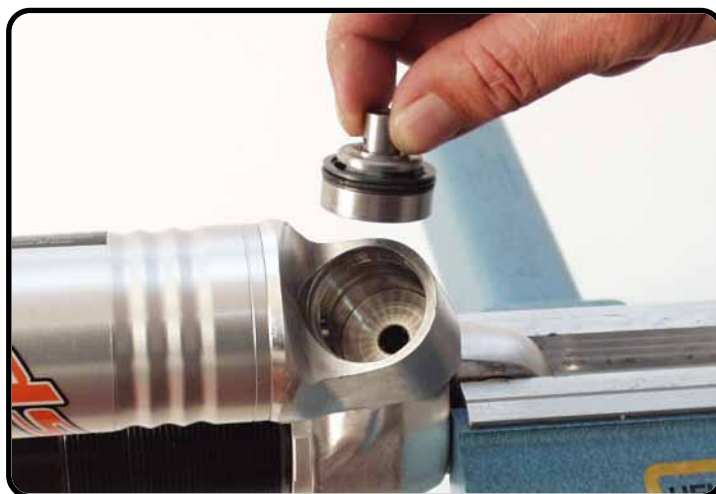
Pull the damping holder "cpl" out of the bottom.
