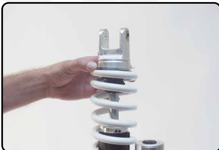
Assemble the second washer.
