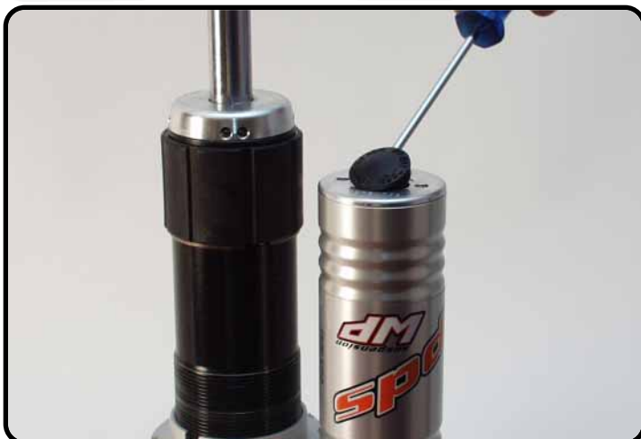
Disassemble the rubber cap.
