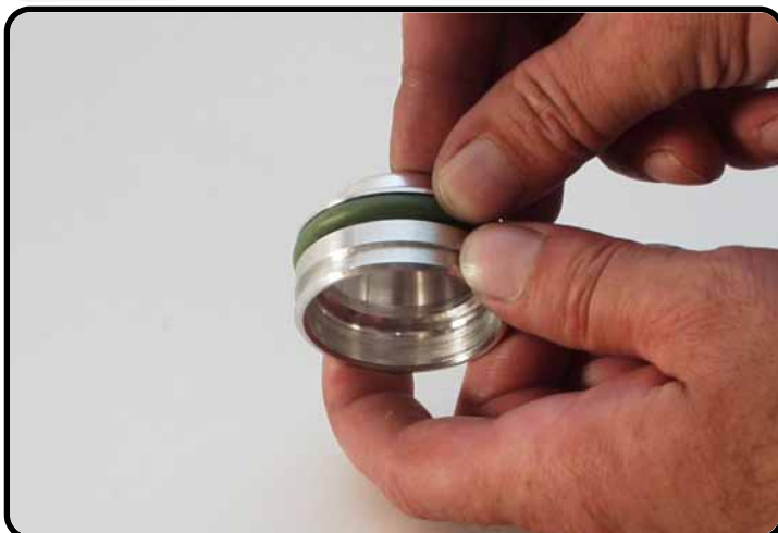
Assemble the O-ring.
