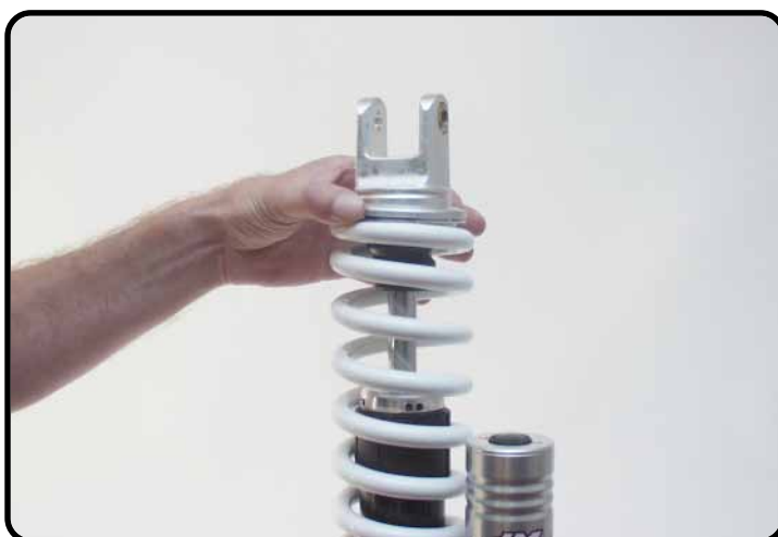
Assemble the spring retainer.
