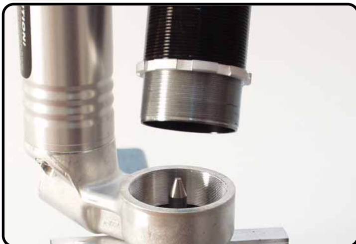
Screw the tube out of the bottom.
