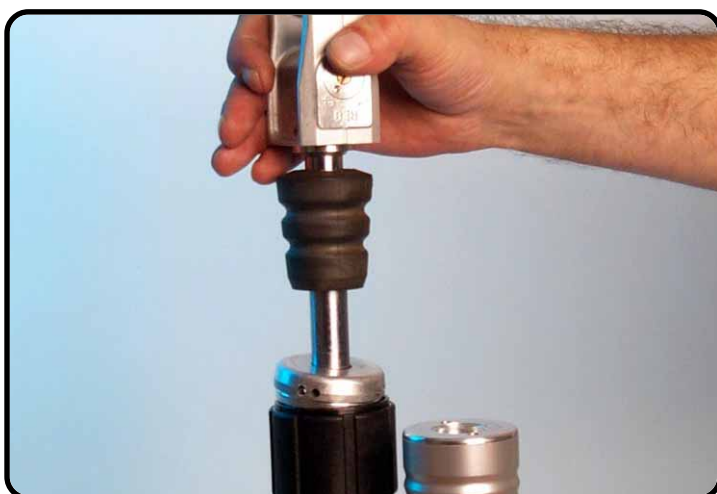
Pull the piston-rod fully out.
