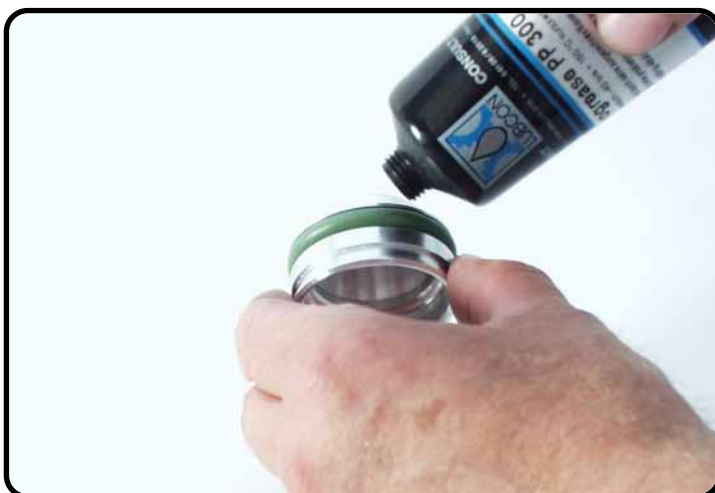
Grease the O-ring with T158.
