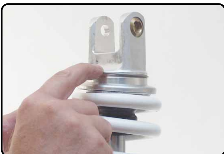
Assemble the springring.
