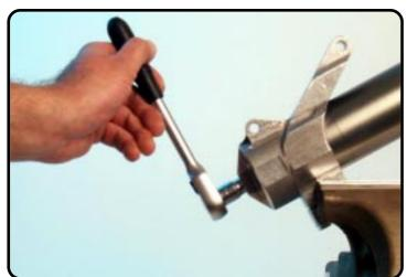
Unscrew the bolt out of the axle-clamp.
