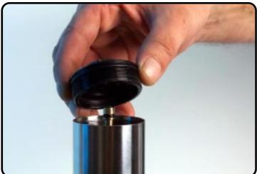
Check the rubber sealing ring inside.
