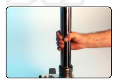
Moving the inner-tube 'not too high', up and down.
