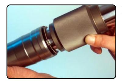
Tapping the dust wiper into the outer-tube.
