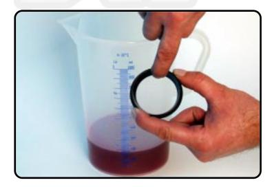
Grease the innerside of the dust wiper with frontfork oil.
