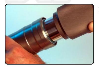
Assemble the oilseal with the other side of T902 into the outer-tube.
