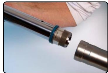
Pull with both hands the inner- out the outer-tube.
