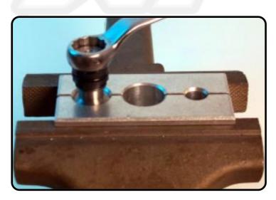
Remove the check-valve nut.
