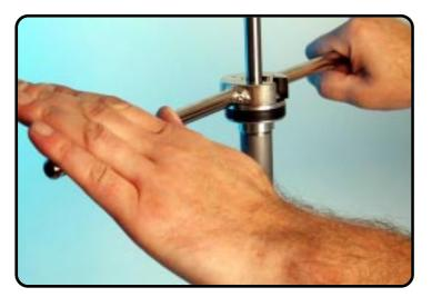
Tighten the screw-cap.
