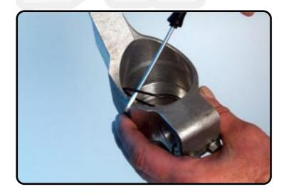
Lift the O-ring out the groove of the axleclamp.
