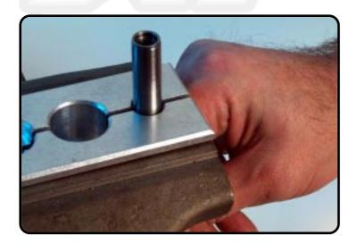
Clamp the piston-rod with the bevelled edge on top in the clamping block.
