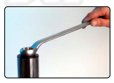
Disassemble the screw-cap.
