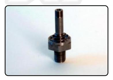
Assemble the shim for checke-valve, piston and rebound shims.
