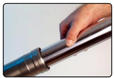
Slide the inner-tube slowly in the outer-tube.
