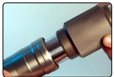
Tapping the DU-bush into the outer-tube.
