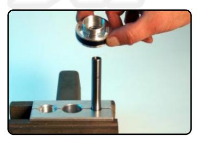
Remove the screw-cap.
