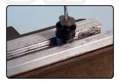
Place a screwdriver on top of the rod tap and remove the entire shim packet.
