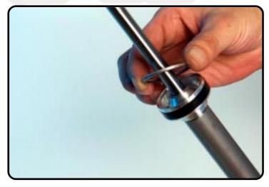
Remove the steel washer. Pay attention to the assembling direction!!!
