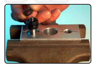
Remove the shim for check-valve.
