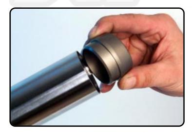
Place T901 on top into the inner-tube.
