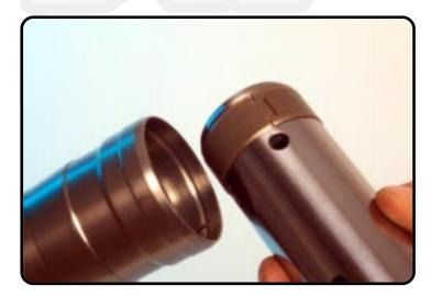
Assemble the DU-bush on the innertube and clamp the (axle-clamp) outertube in the vice.
