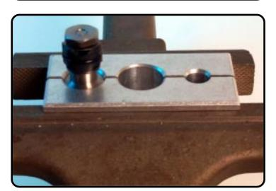
Clamp the tap compression in the clamping block.
