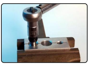
Tighten the check-valve nut to a torque of 5Nm.
