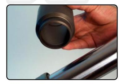
Use T902 -flat side- to tap or push the DU-bush in the outer-tube
