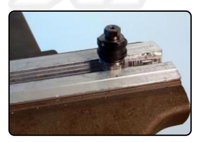
Unscrew the nut. (size 10) Pay attention to the position of the triangular shims and the assembling direction of the nut!!!
