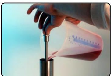
Fill the forkleg with oil just under the edge of the fully compressed inner-tube.
