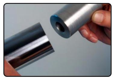
Let inner-tube completely down in the outer-tube and assemble the hydraulic house.
