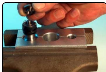
Remove the spring for check-valve. Pay attention to the assembling direction!!!
