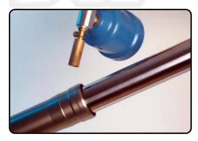
Heat the outer-tube near the oilseal.
