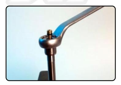
Tighten the piston-rod adaptor.
