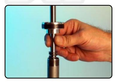
Pull the piston-rod out of the tube.
