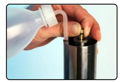
Check the oil level with T137S. Slide the O-ring on level with the edge of the compressed inner-tube.
