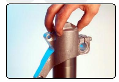
Clamp the outer-tube with T904S inside in the clamping block and assemble the axle-clamp.
