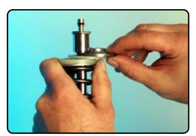
Remove the spring retainer, preload spacers and steel washer.
