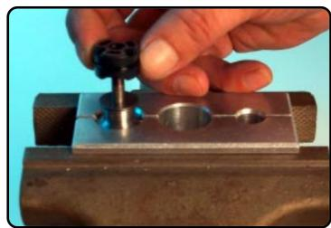
Remove the piston and check the Oring. Pay attention to the assembling direction!!!
