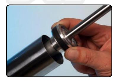
Assemble the cartridge into the forkleg.
