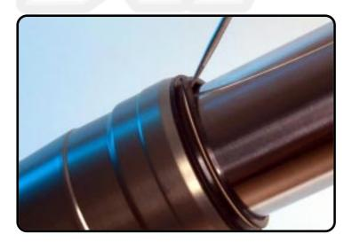
Release carefully the air between the assembled dust wiper and outer-tube with a small screwdriver.
