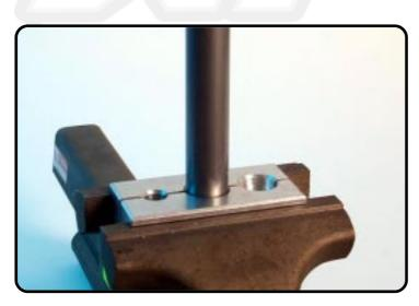
Assemble T907S on the screw-cap.
