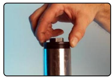
Screw the screw-cap into the innertube.
