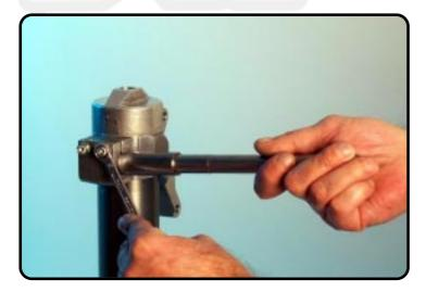
Place a fitting axle-rod in the axle-clamp and tighten both bolts.
