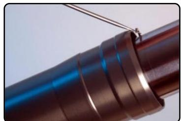
Disassemble the lock washer.
