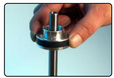
Assemble the screw-cap with steel washer. Pay attention to the assembling direction!!!
