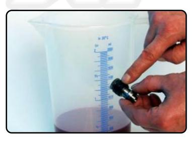
Assemble the tap compression into the tube.
