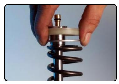
Replace the steel washer and the preload spacers.
