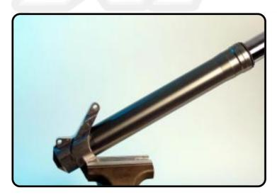
Clamp the axle-clamp in the vice so that the forkleg is about a 45 degrees angle.
