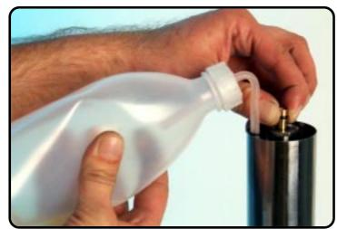
Hold the hexagonal upper side of the piston-rod exactly level with the edge of the fully compressed inner-tube. Also the O-ring of the bottle. Remove the oil till the correct level.
