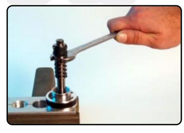
Unscrew the rod tap from the piston-rod.
